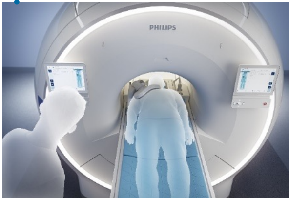
Auto patient centering Region of interest is automatically placed in the iso-center of the magnet
